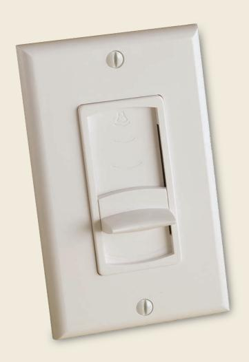
The VLC-100S is an interior decora-style, impedance-matching volume control. Designed to be mounted directly into a standard junction box, the VLC-100S provides a safe operating load to the multi-room audio amplifier and is very easy to operate. A slider-type volume control, the VLC-100S can handle up to 100 Watts per channel and up to 16 pairs of speakers. Five trim colors are included with the VLC-100S: Black, Brown, Almond, Bone and White.
