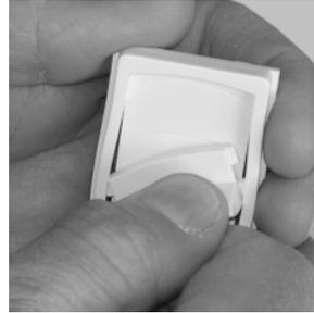
4.) Put the new slide knob into the new faceplate by twisting to the left or right. Some bending is normal and is to be expected.
