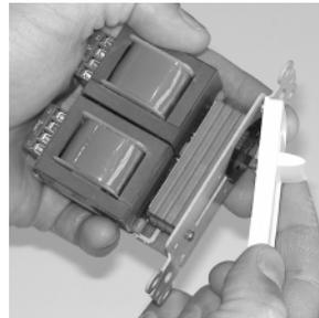
7.) Align the faceplate tabs in the top two holes in the metal back plate. Then, make sure the other two plastic tabs align with the other two holes in the metal back plate.
