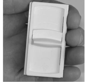
5.) Once the new slide knob is in the new faceplate, check to make sure it slides easily in the slot.
