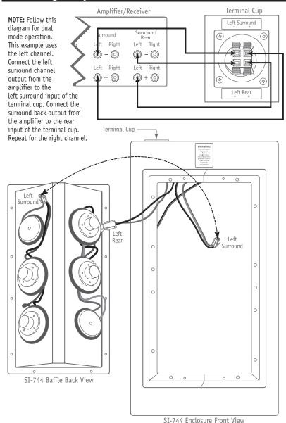
Wiring Diagram 1. Dual-channel operation.
