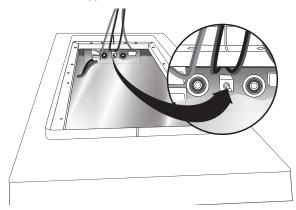
Untape and flip the switch for setup as a single-channel speaker for use in a 5.1 Home Theater (see Wiring Diagram 2 on page 5).
