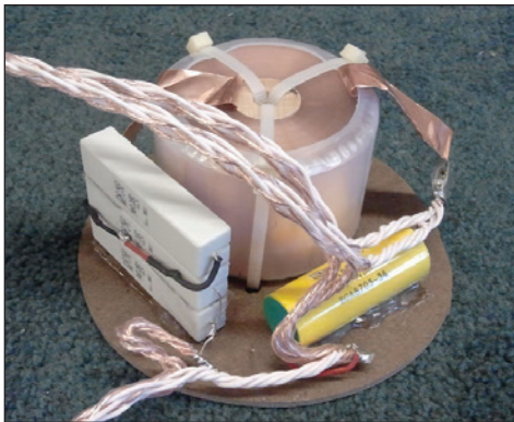
Status Acoustics Crossovers: Tweeter HPF (Top) Midrange BPF (Bottom)
